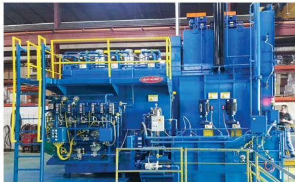
Fig. 2. Integral-quench furnace running the WearAll™ process
